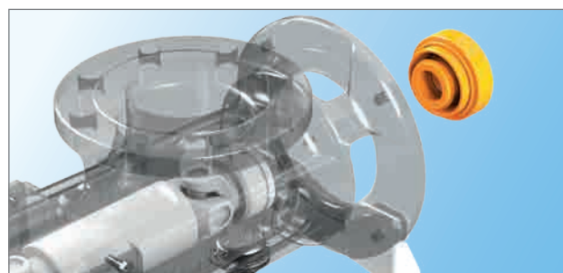
Remove the old seal unit
